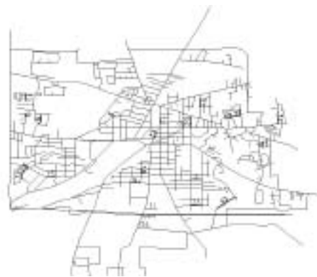
A community map showing the location and ID number of a random two percent of blocksides that can be used to create a random sample inventory.
